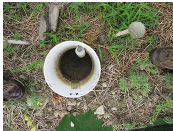
Figure 2. In-ground catchment buckets used to collect leachate from NY cover crop experiment.
