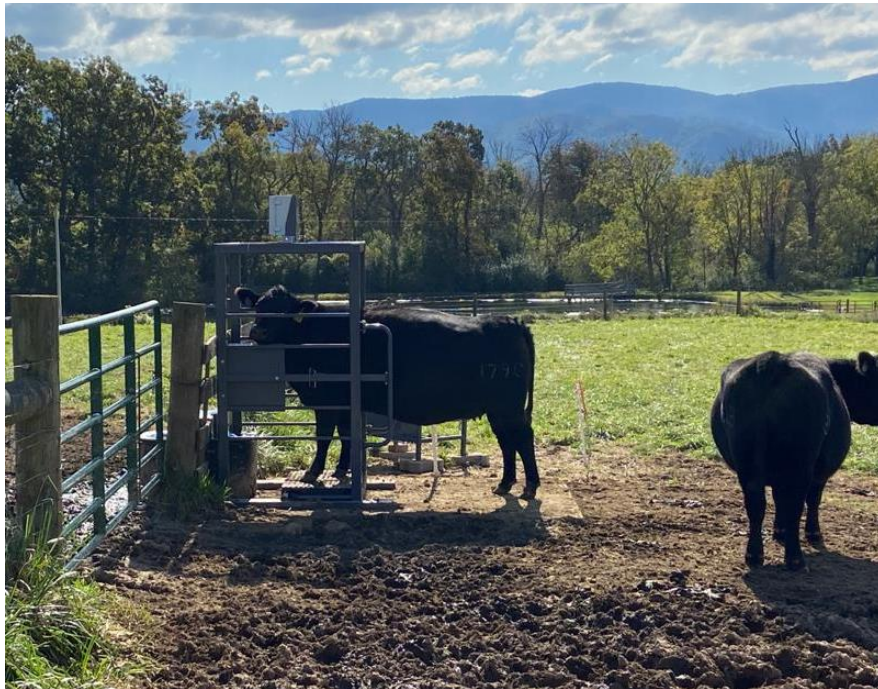
Figure 2: Beef cow being weighed in the SmartScale while drinking water. Notice that only the front legs are on top of the load cells.
